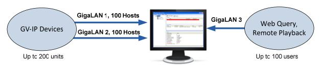
Server installed with GV-Backup Center + 3 Network Cards assigned on different networks
