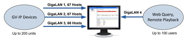
Server installed with GV-Backup Center + 4 Network Cards assigned on different networks
