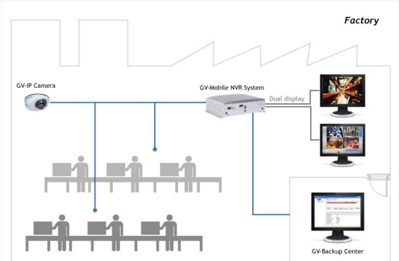
The *GV-MDR220 / 320 / 520 / 1500 Series* are complied with EN50155 and suitable for the installation with GV-Mobile NVR System. With a mobile device or an Internet browser, you can access the live view and recorded events anywhere.
