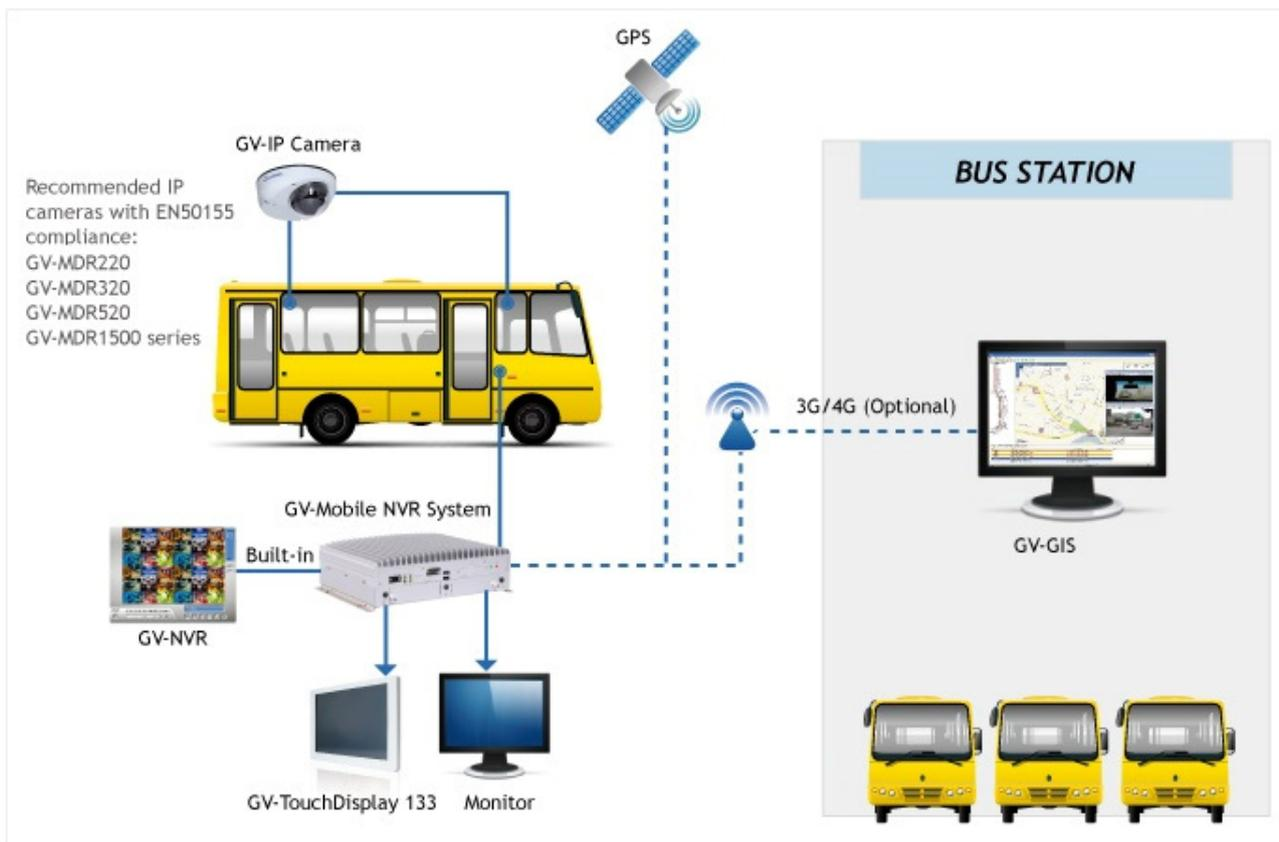
Other than being applied in a public transit, the GV-Mobile NVR can be installed in a fixed and harsh place, such as a factory. In addition, the automatic video backup for the GV-Mobile NVR is made possible by the LAN connection with GV-Backup Center.
